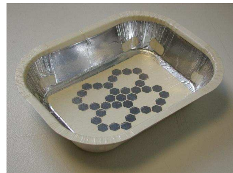
Fig. 15. Food package design with open-circuited antenna base pattern.
