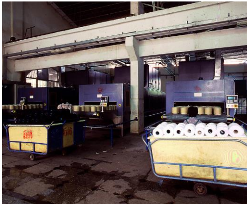
Figure 8 Textile package drying with RF (Courtesy of Strayfield International, UK)
