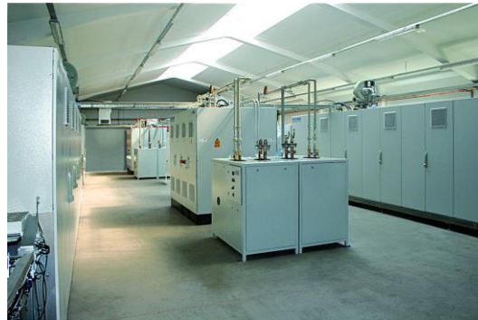
Figure 3 Microwave and hot air dryer for speciality chemicals (With kind permission of Cober Electronics Inc., USA)
