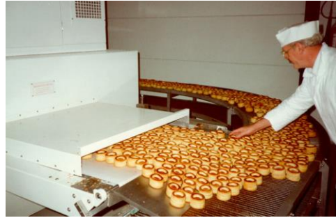
(a) (b) Figure 10 Post baking of vol-au-vent type of product using RF (Courtesy of Strayfield International, UK)
