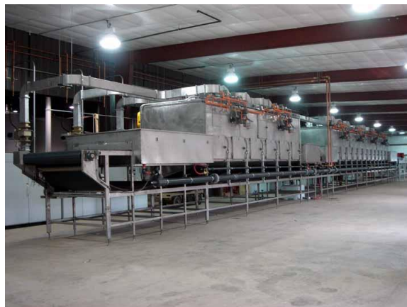
Figure 2 Microwave and hot air combination dryer for sludges (Courtesy of Nemeth-Group Inc USA).
