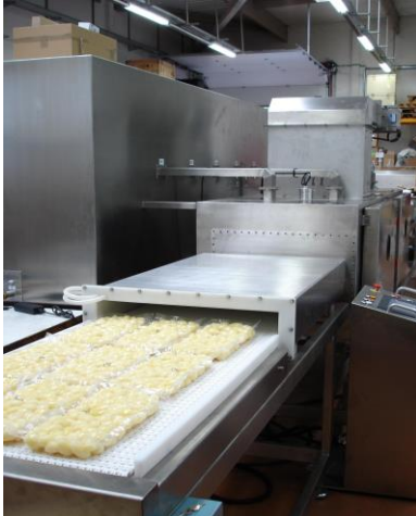
Figure 5 Typical 2.45 GHz pasteurization tunnel (24 or 48 or 76 kW) for fruits, vegetables and ready made meals (Courtesy of Sairem, France)
