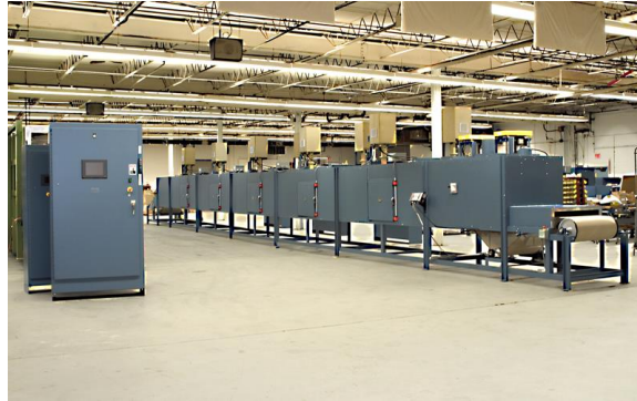
Figure 3 Microwave and hot air dryer for speciality chemicals (With kind permission of Cober Electronics Inc., USA)
