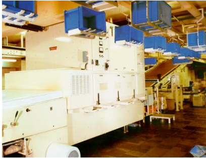
(a) (b) Figure 10 Post baking of vol-au-vent type of product using RF (Courtesy of Strayfield International, UK)
