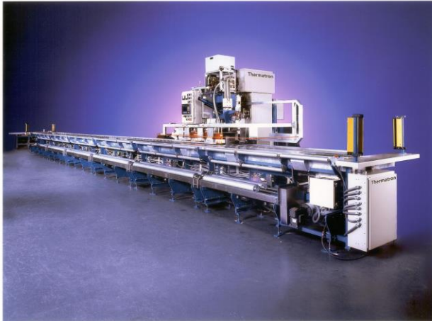
Figure 12 The Travelling Welder for a reinforced industrial fabric (Courtesy of Thermex-Thermatron Inc USA)
